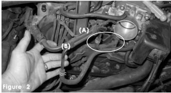
Remove the stock air intake box and stock air intake duct. For this installation remove the all of the PCV hard piping along with the stock lines (B). The only line that will remain is the coolant hose connected to the throttle body port (A).
