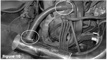
Press on end of the 17mm Injen hose over the ventilation vacuum port and the other end over the large port on the intake.
