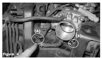
Short coolant hose that will remain intact at the throttle body. Point (A) will be connected to point (B).
