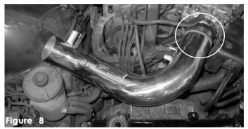
Press the intake into the 2 3/4" hose on the throttle body. Semi-tighten the clamp on the intake side at this point.
