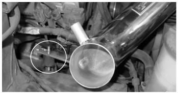
Line up the bracket on the intake to the vibra-mount stud and use the m6 flange nut and fender washer to hold the intake in place.
