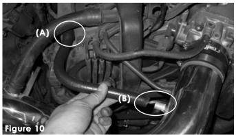
Take the 10mm Injen hose and press one end over the crankcase port (A) and the other over the  $1/2^{\circ}$  port on the intake (B)
