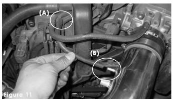
Take the 4mm hose and press one end over the hard pipe vacuum port (A) and the other end over the small port on the intake (B).
