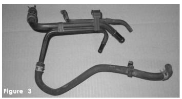
Complete PCV hard piping and stock hose removed from the engine compartment.
