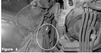
The vibra-mount is screwed in place on the bracket to the side of the fender.
