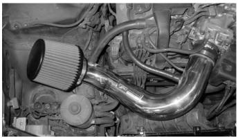
Press the Injen filter over the end of the intake and tighten the clamp on the filter neck. Align the entire intake system for best fit. Once the intake has been aligned and checked for any air leaks, continue to tighten all nuts, bolts and clamps.
