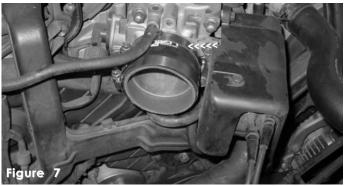
Press the 2 3/4" straight hose over the throttle body and use two clamps, tighten the clamp on the throttle body at this point.
