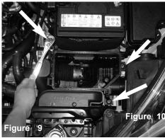
Use a 10mm socket, rachet and extension to remove the three 10mm bolts on the lower air box assembly indicated by the arrow.
