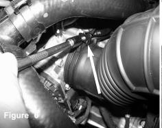
Use a 10mm socket/ratchet loosen the clamp in the throttle body.
