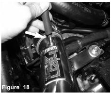
Secure the crank case line to the new intake tube fit-
