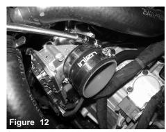
Install the step hose with clamps provided to the throttle body. Tighten the clamp on the throttle body using 8mm nut driver.
