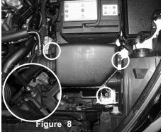
Locate the 3 screws holding in the Factory air box. Loosen and remove using 10mm socket/ratchet.
