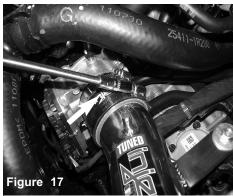
Tighten the remaining clamp on the step hose using 8mm nut driver.
