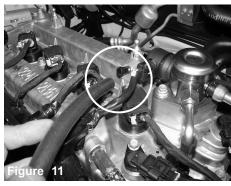
Install the new 8mm hose to the crank case fitting.
