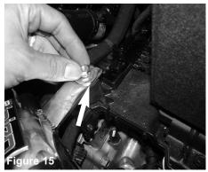
Secure the bracket using provided M6 nut and washer.
