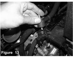
Install the vibra mount to the factory thredded fitting where the air box mounted too. Secure and tighten.
