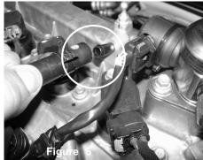
With pliers, press the clamp and pull out the crank case line from the engine fitting.
