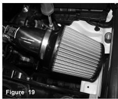
Install the air filter and tighten using 8mm nut driver.
