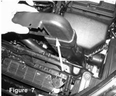
Push the clips holding in the factory scoop. Pull out and remove the factory scoop.
