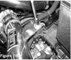
Position for best possible fit. Tighten using 10mm socket/ratchet
