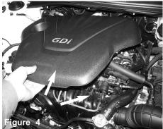
Carefully lift up and remove the engine cover.
