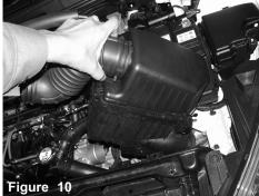
Now carefully lift up and remove the complete air box assembly from the vehicle.
