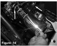
Now install the intake tube and position the intake tube to the throttle body and the bracket to the vibra mount.
