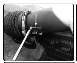
**13.** With T20 torx bit, loosen and remove the 2 screws holding in MAF sensor and remove.
