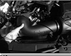
**19.** Place the Injen intake tube onto the throttle body and twist lock filter. Adjust the tube for best fitment and then secure the clamps.
