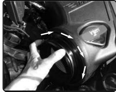
**16.** Once seated, Secure the twist lock filter by rotating in either direction 1/4" turn untill filter locks into place.
