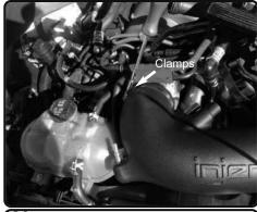
**20.** Adjust the tube for best fitment and then secure the clamps.
