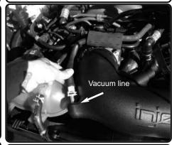
**21.** Reconnect the vacuum line to the 3/8" fitting.
