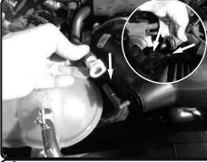
**4.** Disconnect the vacuum line from the intake tube. Pull back the crank case line and sound tube line away from the intake tube.
