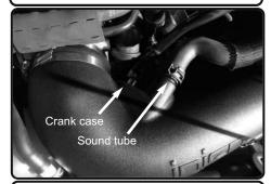
**22.** Reconnect the crank case line to the 5/8" fitting. Re-connect the sound tube and secure.
