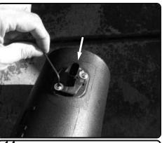
**14.** Now install the MAF sensor into the new injen intake tube using provided M4 screws and secure.
