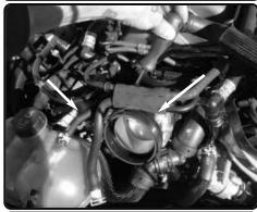
**18.** Install the urethane step hump hose to the throttle with clamps provided and tighten clamp on throttle body only.
