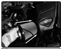
**15.** Install the twist lock filter into the air box.
