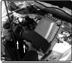
**7.** Now lift up and remove the air box out of the vehicle.
