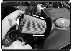
**16.** Install the twist lock filter into the injen air box.
