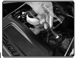
**18.** Re attach the harness to the air box holes on back side.
