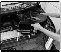
**13.** Install injen air box into vehicle and position to the OEM stand off grommets to chassis.
