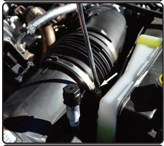
**5.** Loosen the clamp on the airbox using 7mm nut driver.
