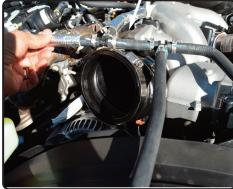
**27.** Install the provided hump hose with clamps to the turbo flange Tighten the clamp on the flange only.
