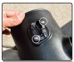
**13.** Install the MAF sensor into the new intake tube and secure using provided M4 button head screws.
