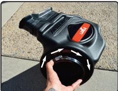
**22.** Once installed and seated, turn in either direction 1/4" turn until filter locks and seats into position.
