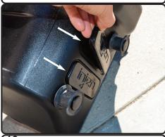
**18.** Optional urethane plugs can be installed to the side of the air box.
