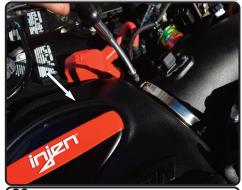
**29.** With provided hump hose and clamps. Attach to the turbo. Install the intake tube.
