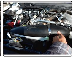
**28.** Install the intake tube into the vehicle, and position tube to filter and hump hose.
