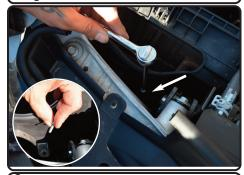
**9.** Locate the screw holding in the airbox, loosen and remove using 8mm nut driver.
