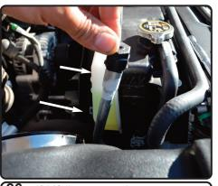
**26.** If A/C line comes close to new injen tube, push forward lightly towards front of the vehicle allowing for clearance.
