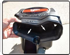
**20.** Push down and make sure the grommets are seated.
