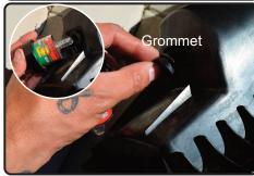
**12.** Carefully pull out the filter monitor and remove the OEM grommet and will be used on the new intake system.
