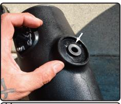
**14.** Install the OEM grommet from step 12 into the hole on the intake tube.
