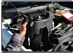
**10.** Now carefully lift up and remove the bottom half of the air box out of the vehicle.
