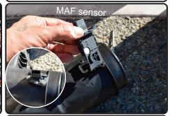
**11.** Loosen the 2 screws holding in the MAF sensor using T20 torx bit and remove.
