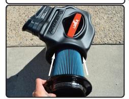
**21.** Install the air filter into the air box.
