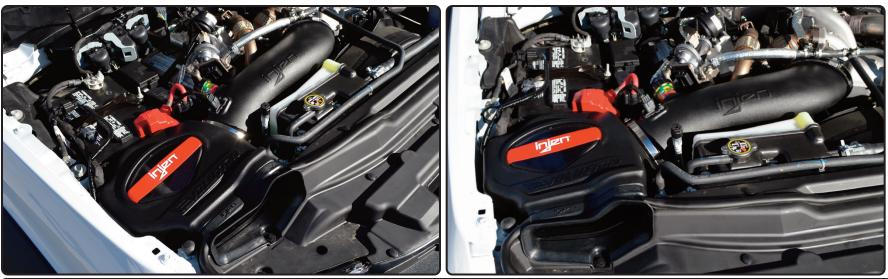
Congratulations! You have just completed the installation of this intake system. Periodically, check the alignment of the intake, normal wear and tear can cause nuts and bolts to come loose. Note: Check clearance and adjust if needed! Failure to check the alignment and adjust the intake can cause damage that will void the warranty. Injen Technology is not responsible for any damages caused by/from improper installation.
