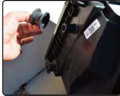
**16.** Remove the Rubber O rings from the OEM air box.
