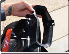
**19.** Install the rubber inlet duct to the front of the air box. Locate the 2 rubber studs to the holes on air box.
