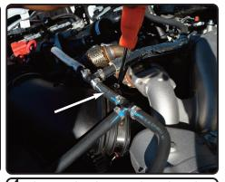
**4.** Loosen the clamp on the turbo using 7mm nut driver.
