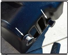
**17.** Re-install into the new intake system plastic fittings.
