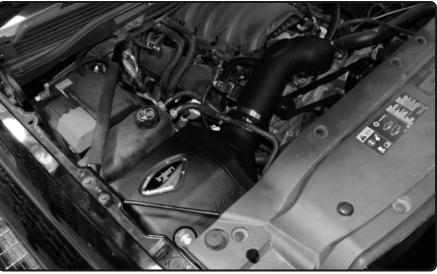
Congratulations! You have just completed the installation of this intake system. Periodically, check the alignment of the intake, normal wear and tear can cause nuts and bolts to come loose. <u>Note: Check clear</u><u>ance and adjust if needed! Failure to check the alignment and adjust the intake can cause damage that will void the warranty. Injen</u><u>Technology is not responsible for any damages caused by/from improper installation.</u>
