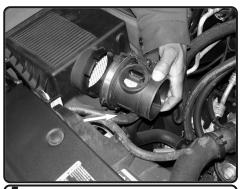
**5.** Loosen the clamp using 8mm nut driver. Remove the MAF sensor from air box. Remove the factory coupler from MAF sensor.
