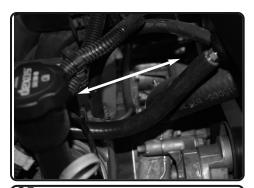
**25.** Install the provided 8mm hose to the crank case vent tube on engine, and connect the other end to the fitting on the intake tube.
