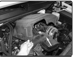
**2.** Pull the engine cover off the intake manifold.
