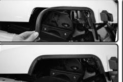
**10.** Place the 16" vinyl trim onto the edge of the cut out. Re-install your hood and the snorkel is ready for installation
