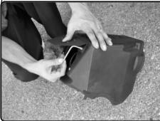
11. Use an allen wrench and remove the Air Box Shield Air Director from the Injen air box. This shield will no longer be used. The snorkle will now be installed.
