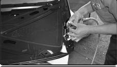
**9.** Use a flat grinder to straighten the edges and clean up all the metal burrs. Slowly grind back on the open. Only grind what you need for additional clearance. Please use caution and have proper safety equipement like goggles and air respirator!!!
