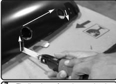
**7.** The line drawn from the template in figure 10 will be a guide to cut using an air saw to cut a straight line. Please use caution and cut slow!!!
