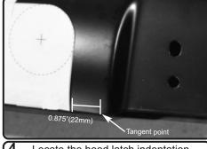
4. Locate the hood latch indentation outer tangent point and measure 0.875" left of tangent to locate supplied cutting template.
