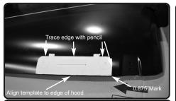
**5.** Now tape the cutting template to the hood from the 0.875" mark from figure 9 and make sure you line up the bottom of the cutting template to the edge of the hood. Use a pencil and trace the edge of the template for a cutting guide for the next step.
