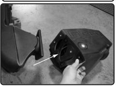
**12.** Place the supplied gasket in between the Injen air box and the snorkel
