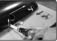
**12.** The line drawn from the template in figure 10 will be a guide to cut using an air saw to cut a straight line. Please use caution and cut slow!!!
