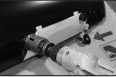
11. Using the crosshairs on the cutting template as a guide, use a 1 3/4" hole saw and drill out the two holes on the template. Make sure you drill past the second layer of the hood. Please use caution!!!
