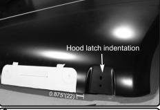
8. Remove the hood from the vehicle. Measure 0.875" (22mm) from the hood latch indentation outer tangent point. Tape the cut template onto the hood. Figure 9 will have a close up of the measuring point
