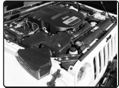
**7.** Injen intake system and air scoop installed.
