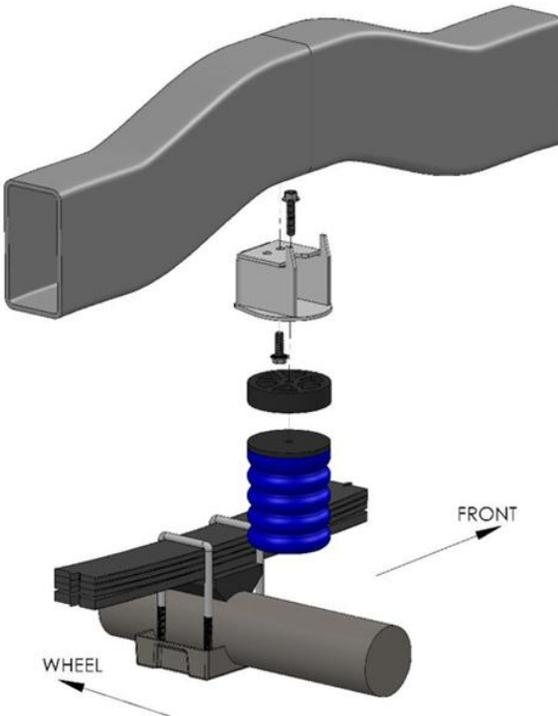
Brackets can be used on either side of the vehicle. On both sides, use forward hole to center SumoSpring over the axle.
