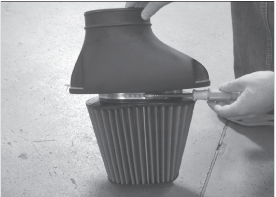
Figure 9- Securing Banks Ram Air Filter Cover to Banks Air Filter
