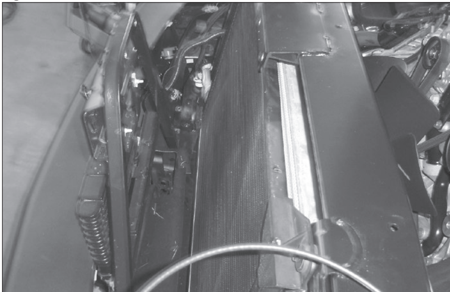
Figure 2.8 Upper Intercooler (CAC) Attachment Bolt.
