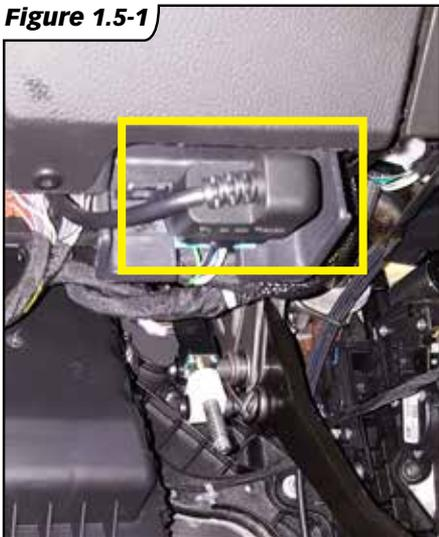
**2.** Route the Starter Cable and OBD-II Cable to the dash.
