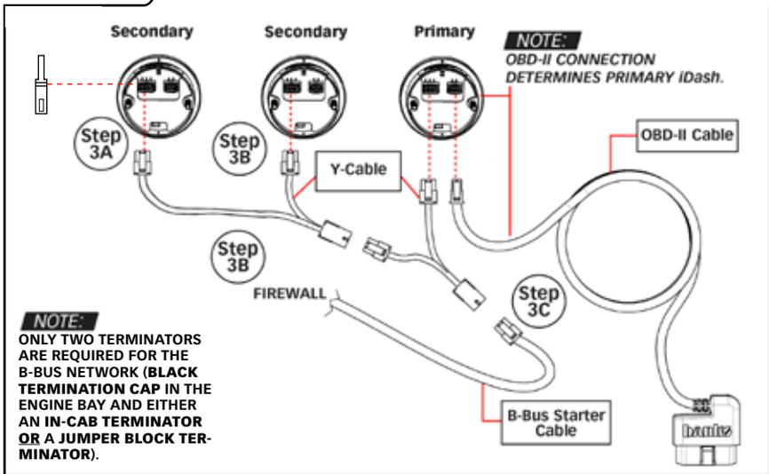
**3.** Connect the Y-Cable to the 6-pin port of the first and second iDash 1.8 (**without the In-Cab Terminator**). See **Figure 1.5-11**
